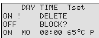
Figure 8.26 Confirm deletion of block from week program
